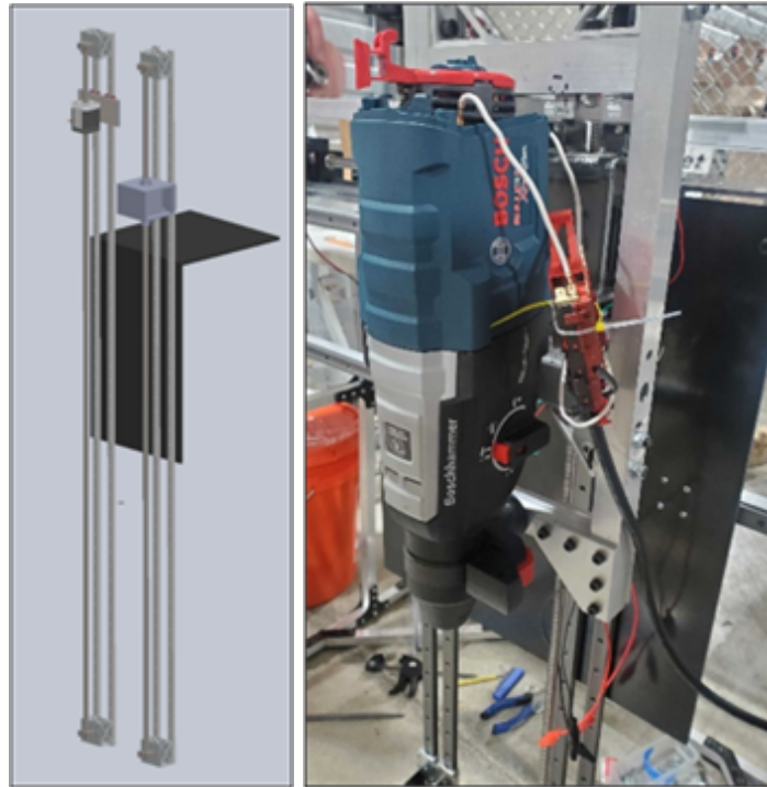
Figure 3a: TAURUS Vertical Traverses. Visual representation of the vertical traverse components mounted onto the sub-platform. The sub-platform is then mounted onto the horizontal traverse system.
