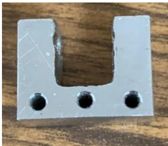
Fig. 12. C section for class 2 joint
