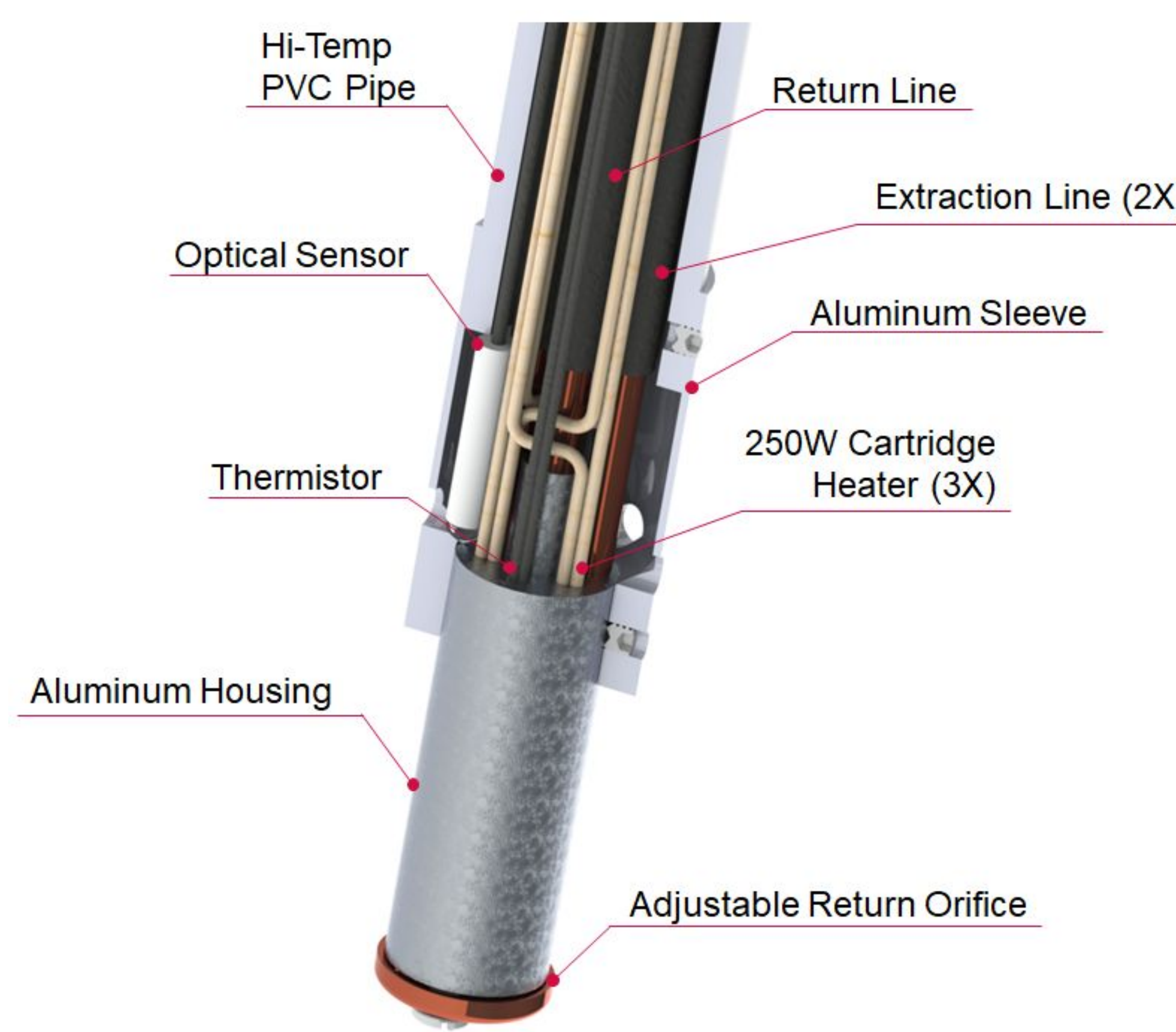
Section View of Extraction Probe
