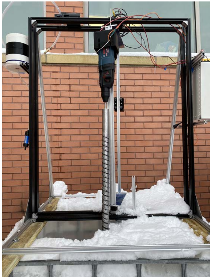
Figure 2. JAMMER prototype mounted on simulated ice box in below -20C outdoor conditions
