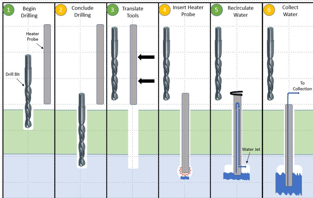
**Figure 2.** Sequence of Operations for STYX & STONES on the Moon and Mars
