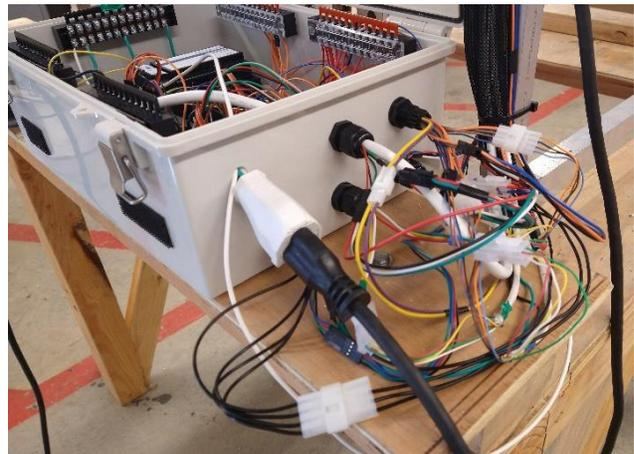
*Figure 9B. Wire disconnects for easy disassembly and transportation*
