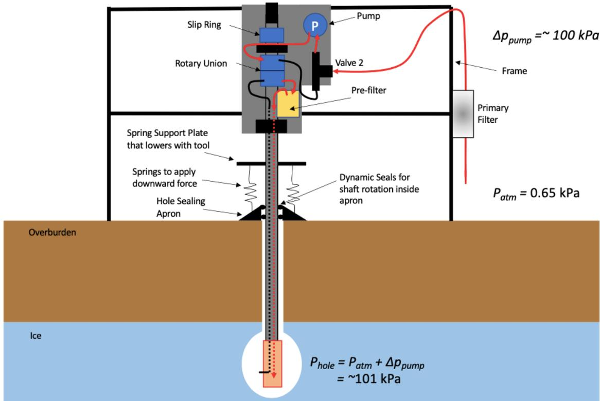
**Figure 10.** Schematic of Hole Pressurization Design Solution
