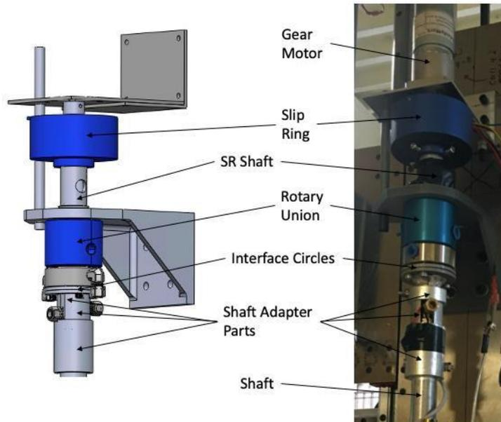
**Figure 6.** Rotary joint CAD model (left) and manufactured subsystem (right)
