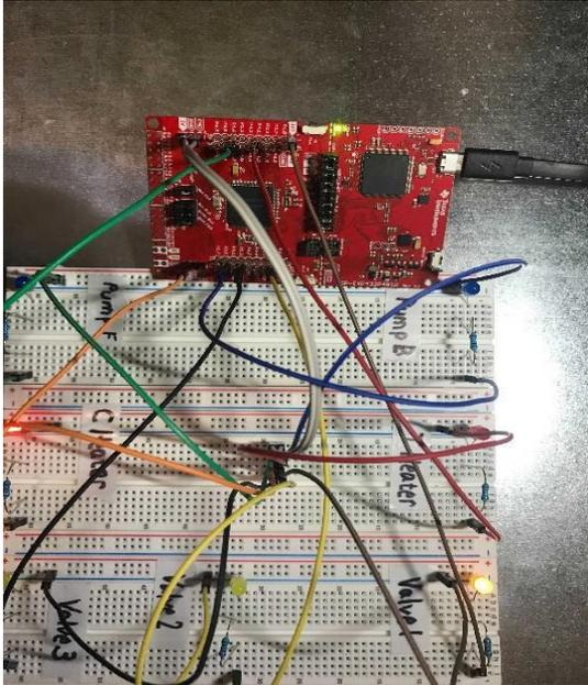
*Figure 7. LED and Breadboard setup to test signals and timing from Microcontroller*
