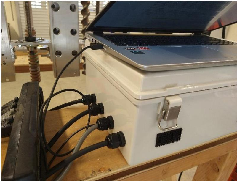
*Figure 8. Microcontroller connected to laptop with micro-USB*
