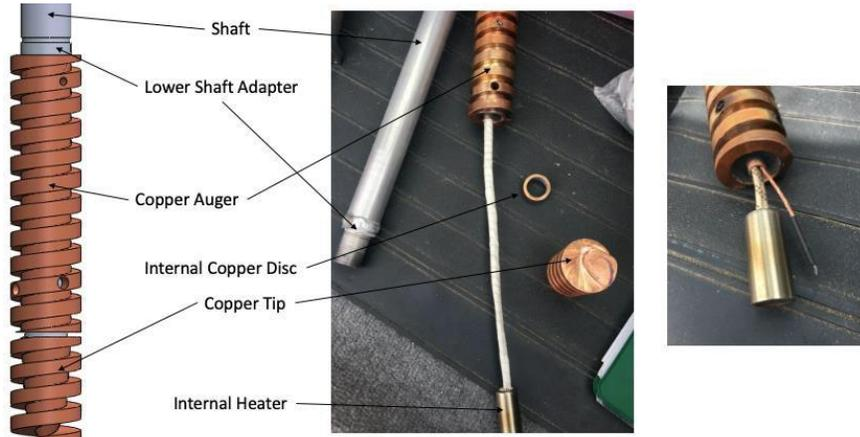
**Figure 3.** Manufactured parts in the Heated Auger assembly
