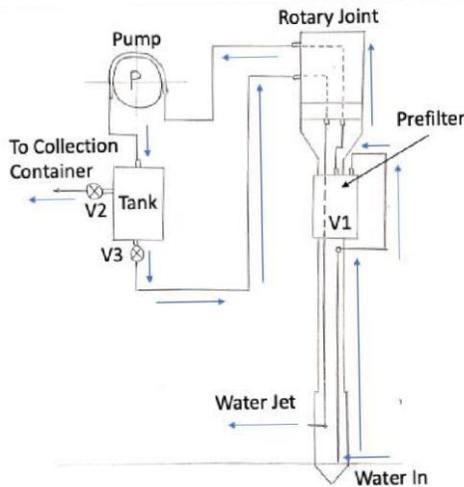
**Figure 5.** Water extraction schematic
