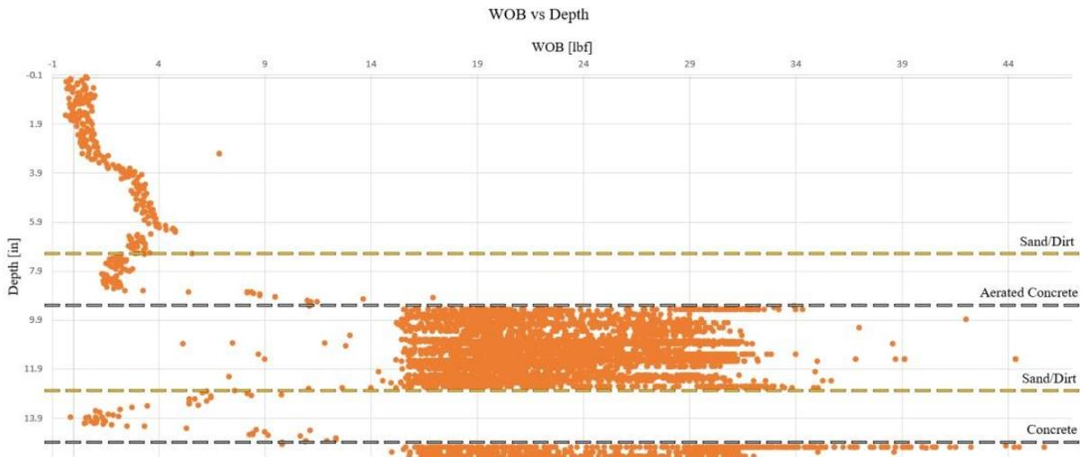
**Figure 4.** Prospecting for Digital Core using WOB Recordings
