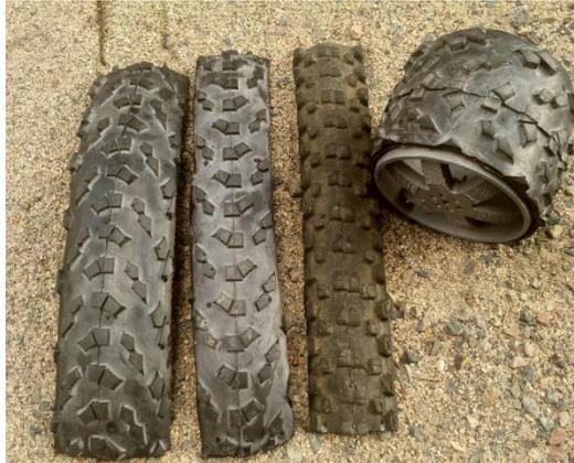
Figure 6: Tread patterns of the two rovers
