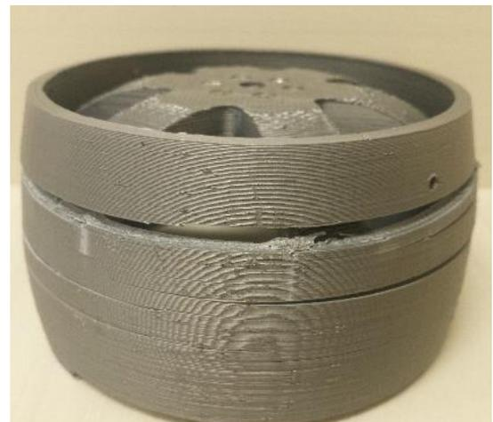
Figure 10: Tested Wheel displaying cracks along the layers of the 3D Printed model.
