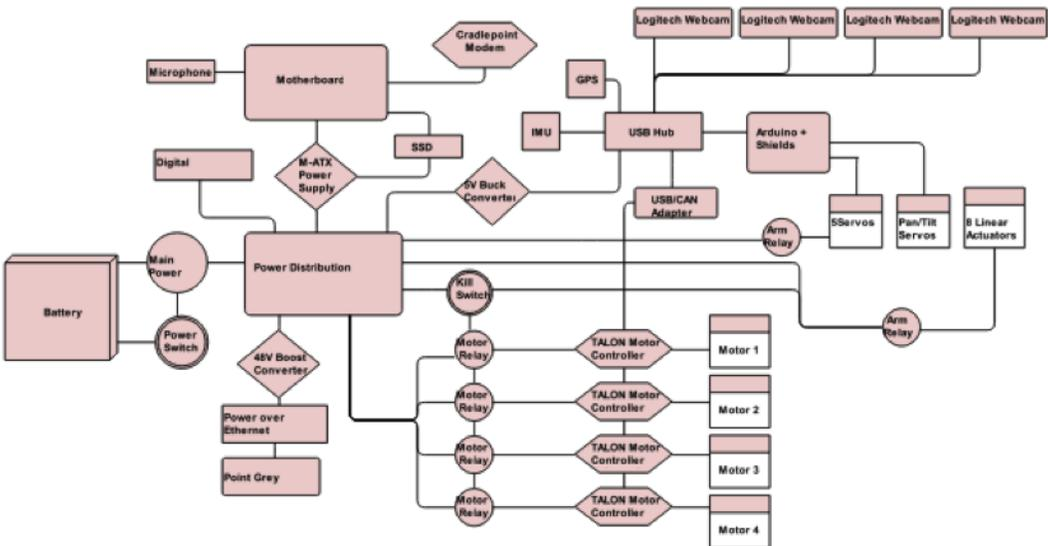
Figure 8: Electronics System Block Diagram
