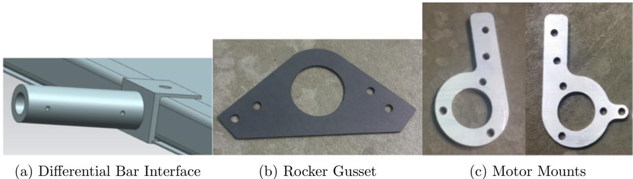
Figure 1: Chassis Components
