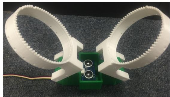
Figure 5: Ultrasonic sensor placed inside the end effector housing
