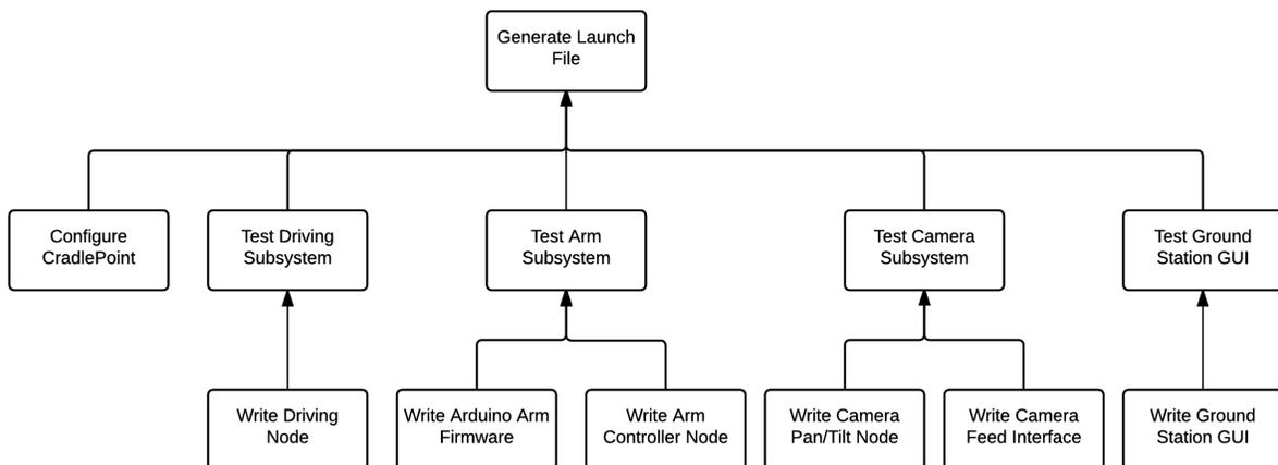
Figure 7: Software System Block Diagram
