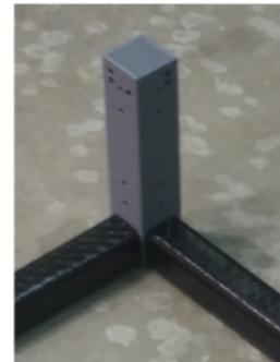
Figure 2: Corner Chassis Piece
