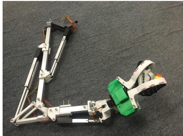
Figure 3: Aluminum Version of Manipulator System
