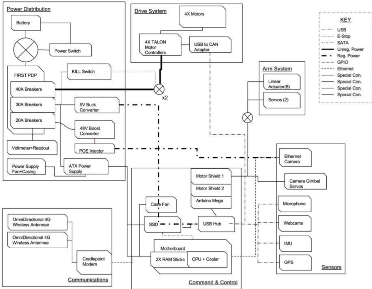
Figure 9: Power and Connections Diagram
