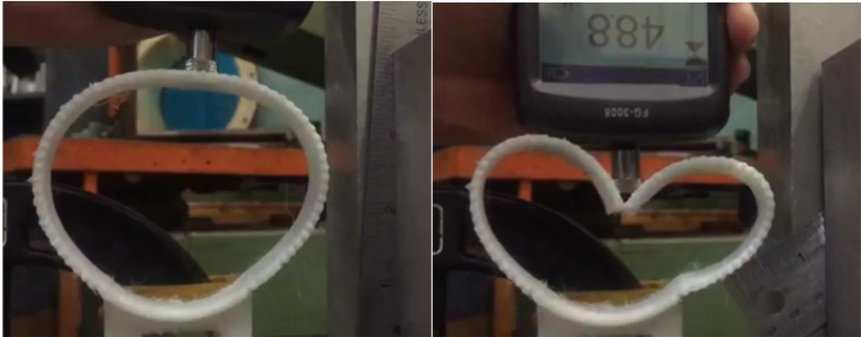
Figure 4: Compression force tests on the primary end effector
