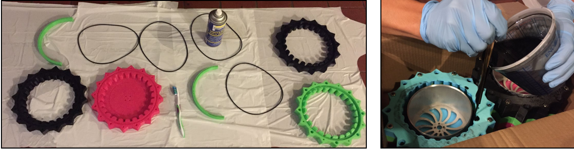
Figure 4: a) Pieces of the wheel mold & b) pouring urethane around the aluminum wheel assembly
