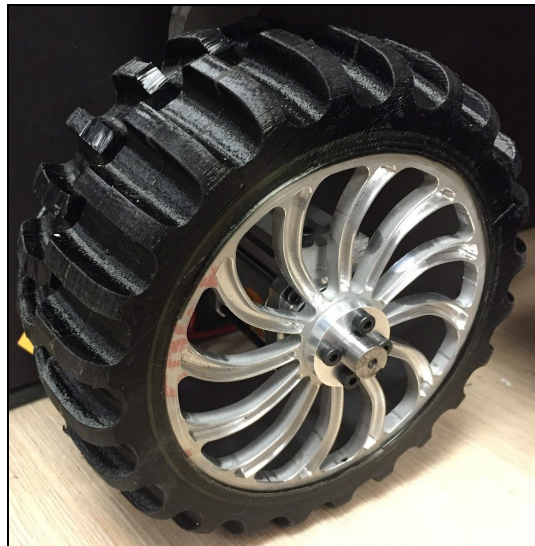
Figure 5: A single completed wheel assembly mounted onto the gearbox shaft
