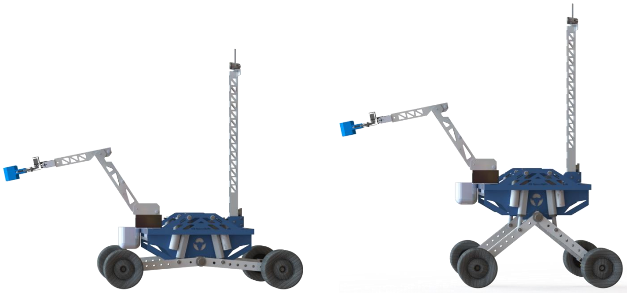
Figure 2: Astraeus III at Minimum and Maximum Suspension Height
