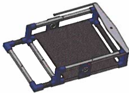
Figure 2.1.1: A CAD model of the rover chassis. Above is the chassis model of the rover Optimus showing the carbon fiber plate, Aluminum and carbon fiber tubes and ABS joints
