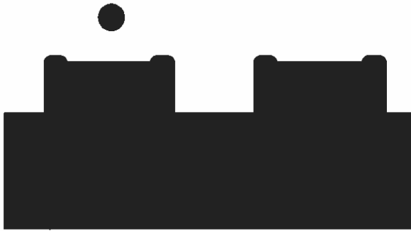
Figure 3: Robot silhouette used for collision detection, with (left), and without (right), an additional obstacle in the workspace.
