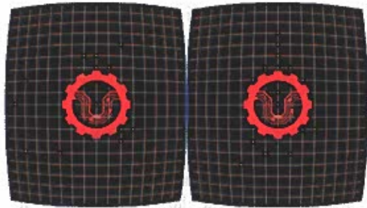
FIGURE 10: AN EXAMPLE OF BARREL DISTORTION AND COLOR CORRECTION FOR A HEAD MOUNTED DISPLAY
