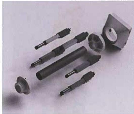
FIGURE 6: EXPLODED VIEW OF THE MODULAR WRIST ASSEMBLY
