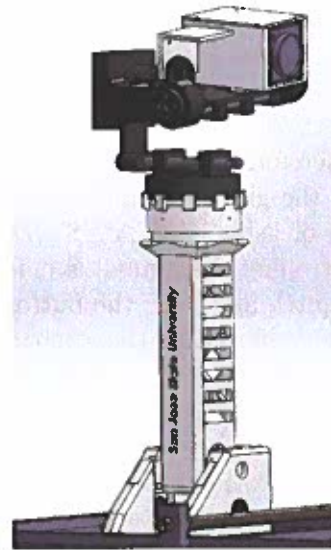
Figure 3: CAD of Camera Gimbal with Camera and Lidar Mounted
