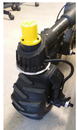
Figure 2: Wheel Assembly using ABS
