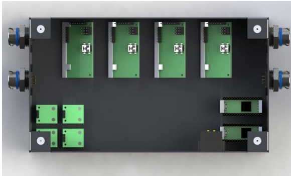
Figure 7: Drive controller box, top view.
