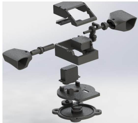
Figure 14: PTS3D, detailed exploded view.
