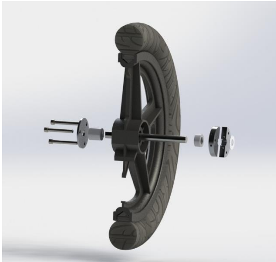
Figure 5: Wheel assembly, detailed exploded view.
