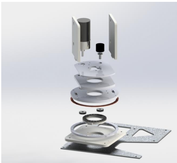
Figure 9: Manipulator arm turntable, detailed exploded view.
