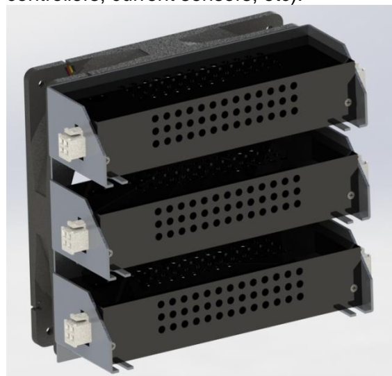
Figure 17: Voltage regulation cluster, detailed view.
