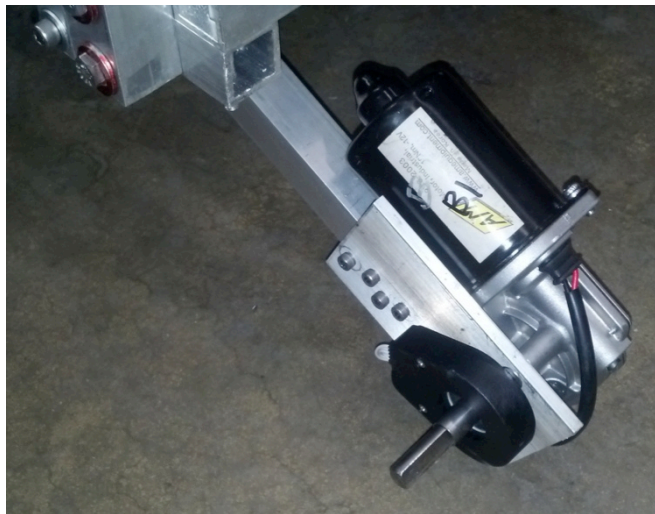
Figure 2. Motors with Attached Encoders
