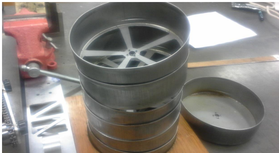
Figure 2: Steel portion of the wheels, mid production
