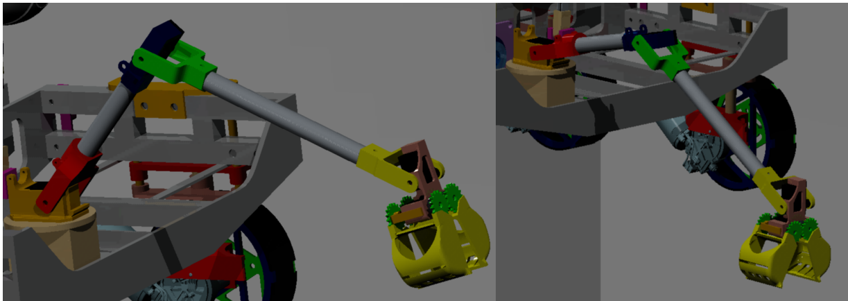
Figure 4 - 3D CAD Model of Arm and Manipulator Sample Retrieval
