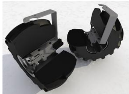
Figure 7: Rubber wheel with in-wheel brushless DC gearhead motor.
