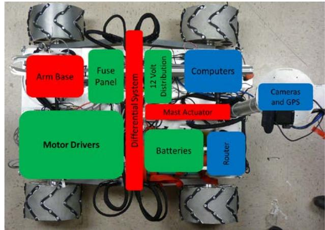
**Figure 12: ROCbot chassis layout.**
