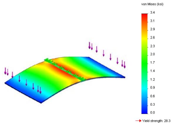
**Figure 9: Chassis plate finite element analysis.**
