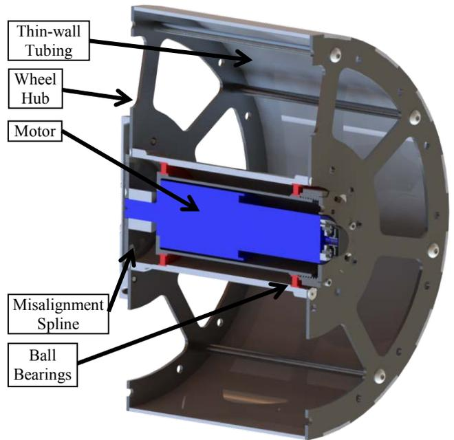
**Figure 6: ROCbot wheel cross section view.**
