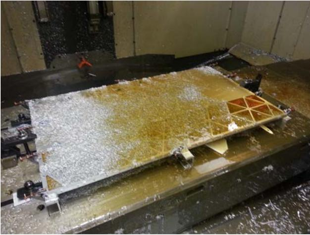
**Figure 10: ROCbot chassis plate in the CNC.**
