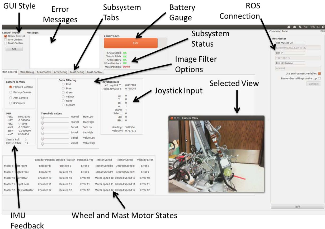
**Figure 19: The main GUI will be split onto two screens for the competition. One screen dedicated to camera views and the other to telemetry.**
