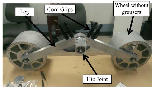
**Figure 5: Right side of the ROCbot suspension.**
