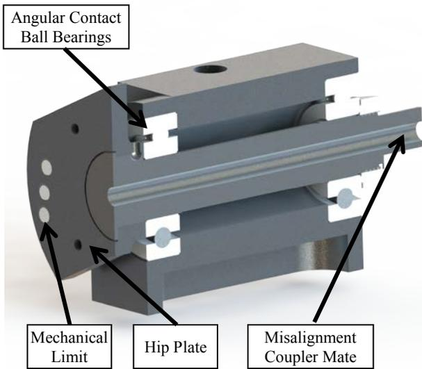
**Figure 3: Cross section view of the hip joint.**
