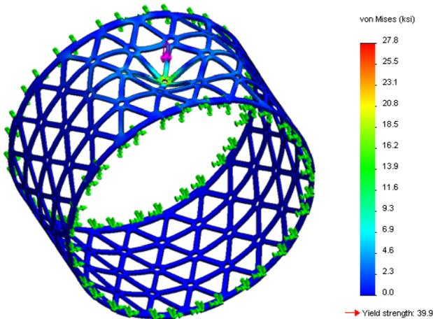
**Figure 8: ROcbot wheel tubing with lattice structure finite element analysis.**
