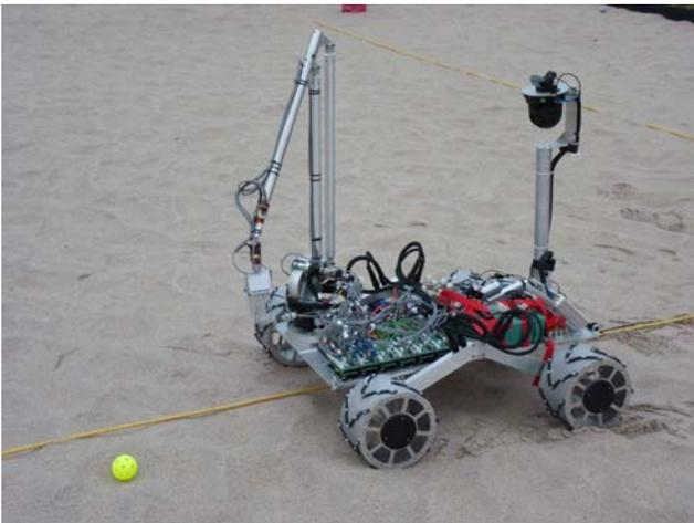
Figure 21: Manual testing in sand.
