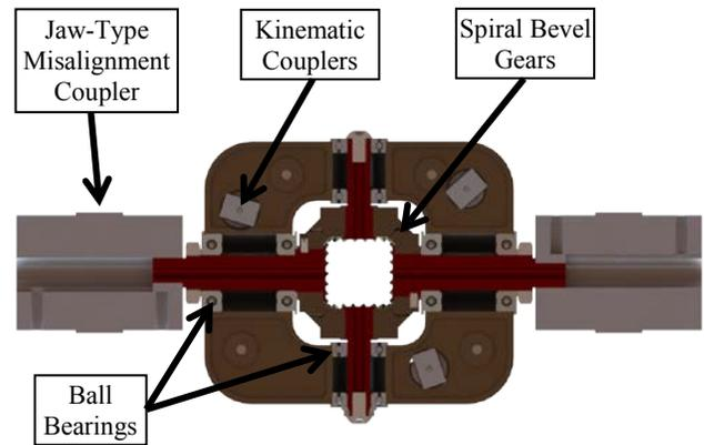
**Figure 2: ROCbot differential averaging system differential bearing block cross section view.**
