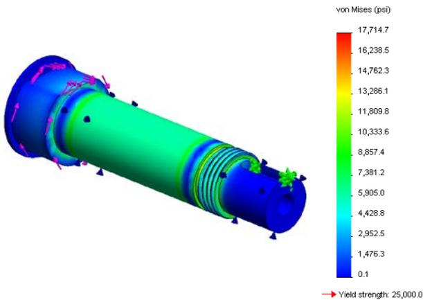
**Figure 4: Differential shaft finite element analysis.**
