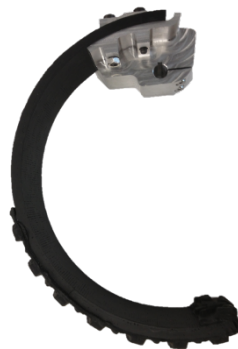
Figure 1: Fiberglass leg with tire tread and two-piece aluminum clamp
