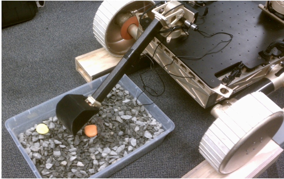
Figure 10: Testing the Arm Payload on Gravel
