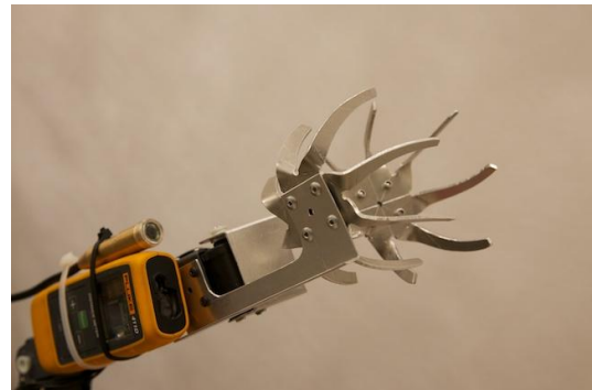
Figure 10: Sample Acquisition Arm End Effector
