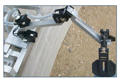
to rotate. The rotation of the plate is driven by another servo that is mounted underneath it and the plate itself is mounted to the sub-frame of the entire rover. Towards the base of the arm, another servo holds the spool that will draw the aircraft cable in and out to operate the clamp mechanism.
