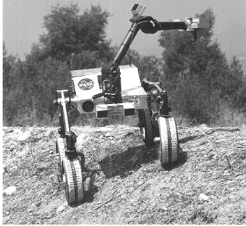
Figure 5 Articulated Suspension (Courtesy: NASA)
