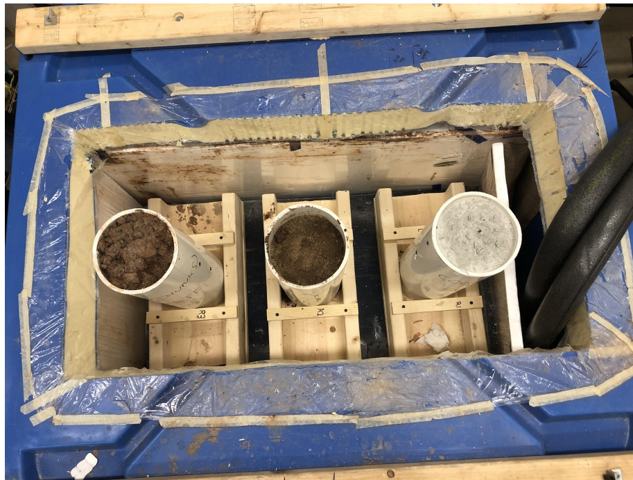
Figure 5: We created three different layered cores for use during integration testing, in order to assist with the development of digital indicators for the interpretation of layers at the competition. The cores are easy to lift and remove / replace and give access to the ice below in order to allow “post mortem” examination of each drilling experiment.
