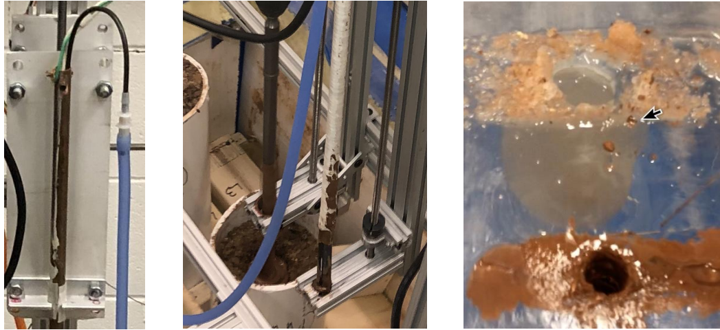
Figure 3(a): Mounting plate for heater and water inlet assembly, 3(b): Restraining bushings for drill bit and heater assembly, 3(c): Spherical 1.4 liter ice cavity melted by radiative heater and filled with dirty water.
