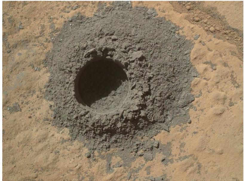
**Figure 8: Hole Drilled on Windjana by Curiosity on Mars**
