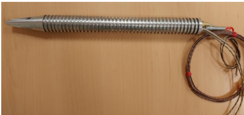
Figure 7: MIDAS Extraction System
