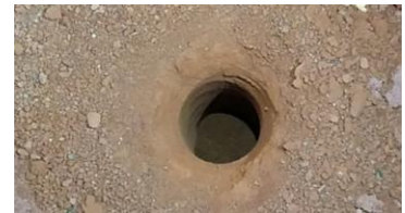
Figure 9: MIDAS Drill Test on a Loosely Packed Frozen Sample
