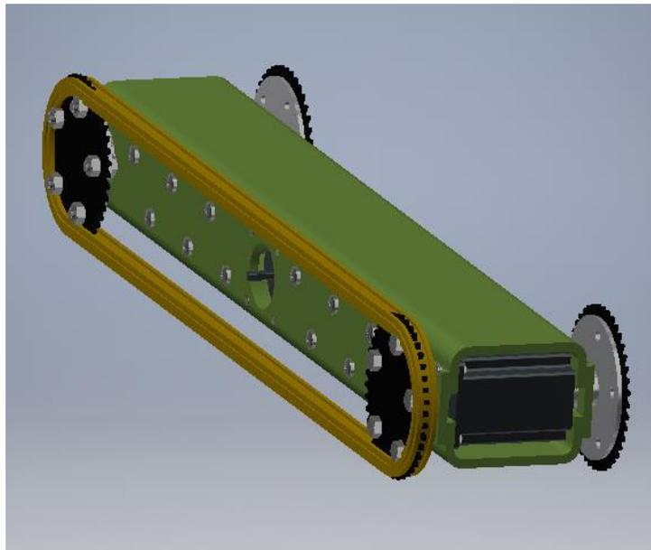
**Figure 2:** Trencher Unit with Teeth and Second Chain Removed
