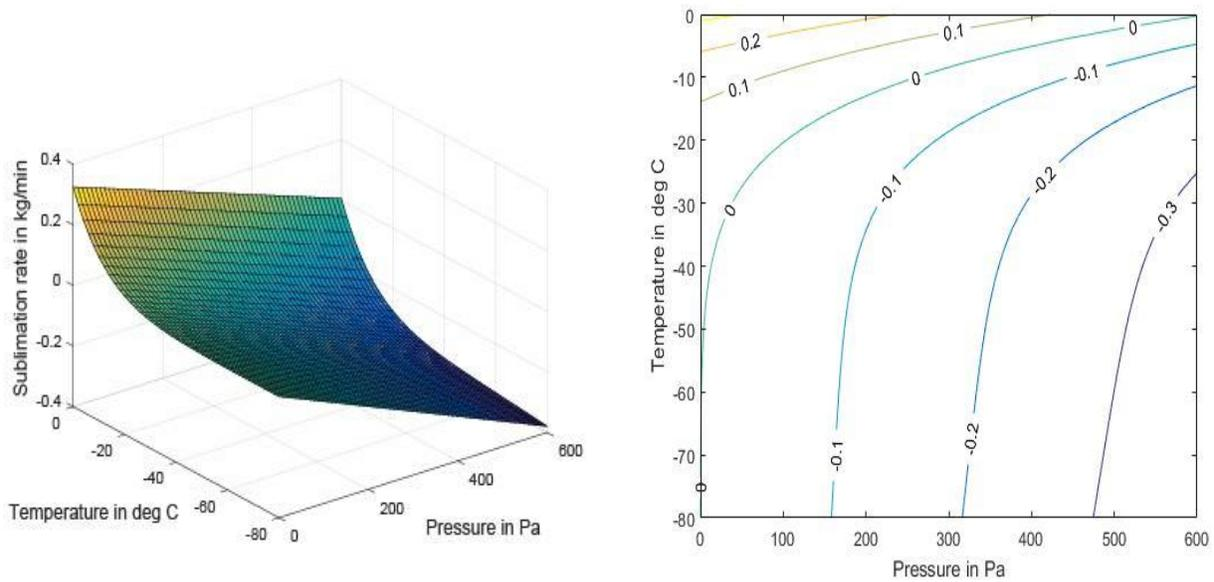
**Figure 6:** Sublimation Rate over a Range of Temperature and Pressure
