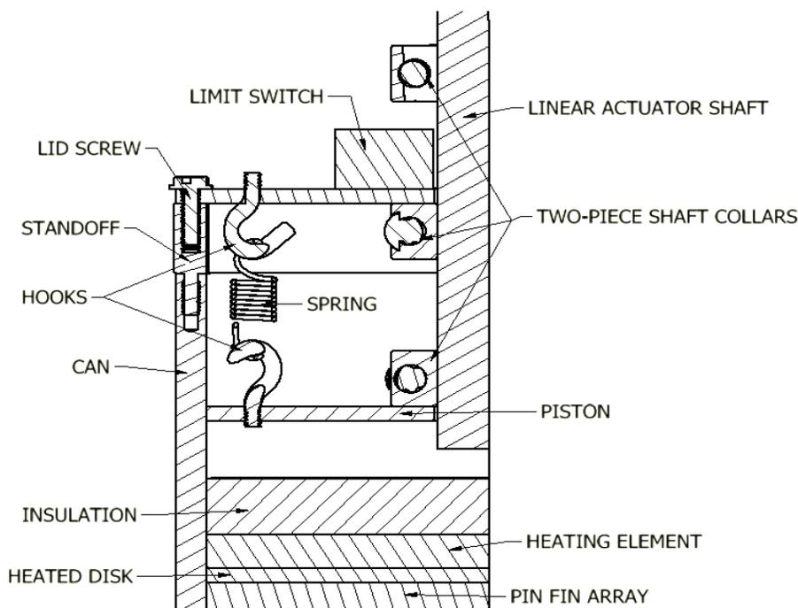
**Figure 3:** Cross-Section of Extraction Can
