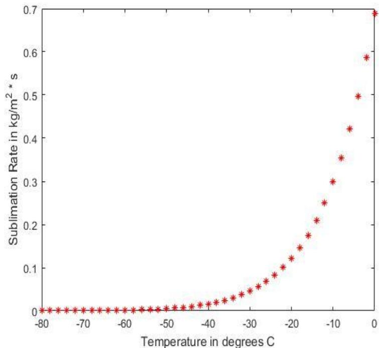
**Figure 8:** Sublimation Rate as a Function of Temperature for a 10 cm Diameter Unit in a Vacuum
