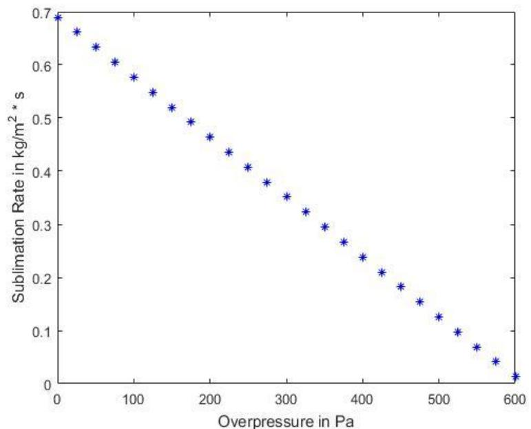
**Figure 9:** Sublimation Rate as a Function of Pressure for a 10 cm Diameter Unit
