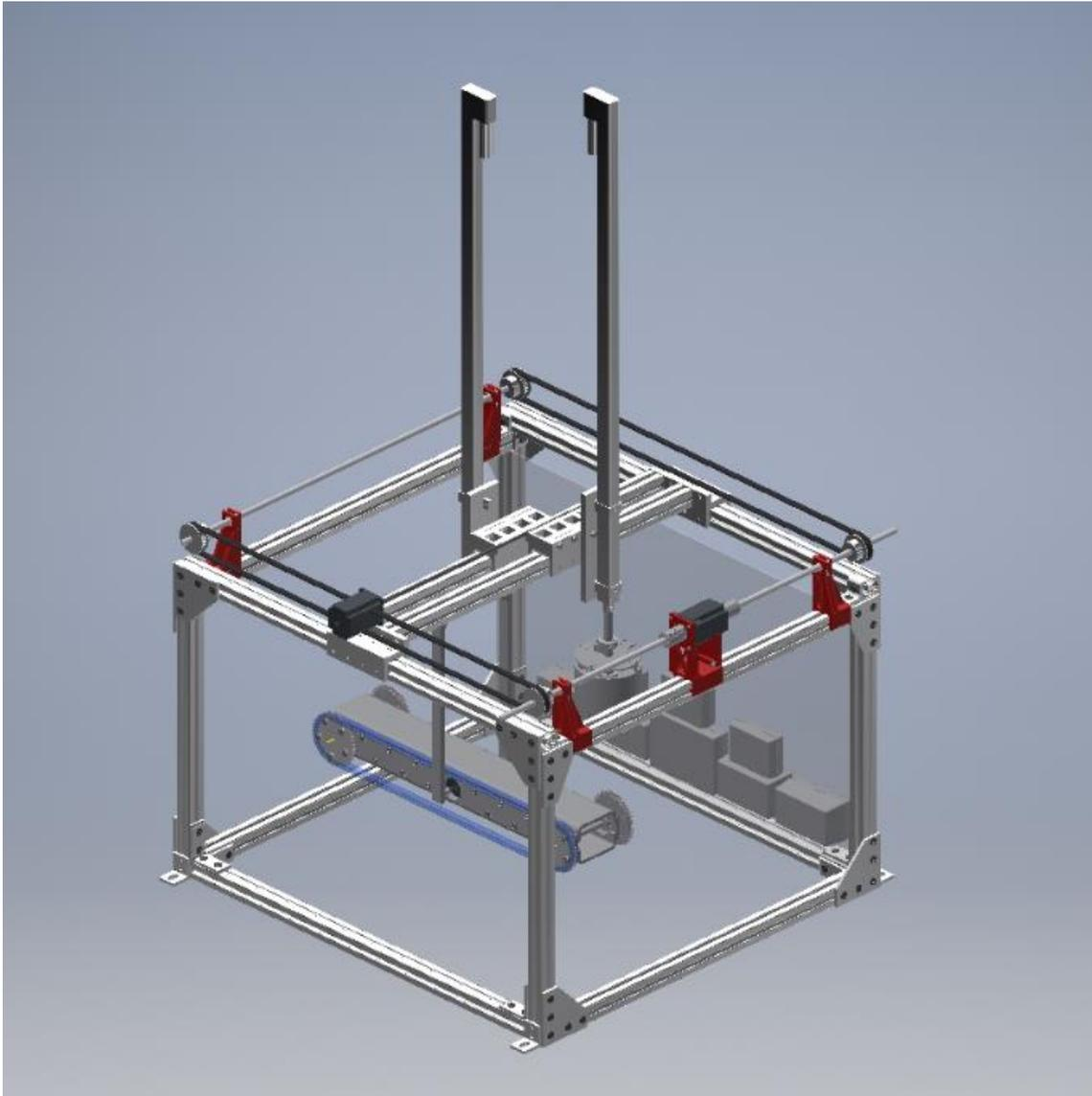
**Figure 1:** Model of 3-Axis Gantry System with Linear Actuators Attached
