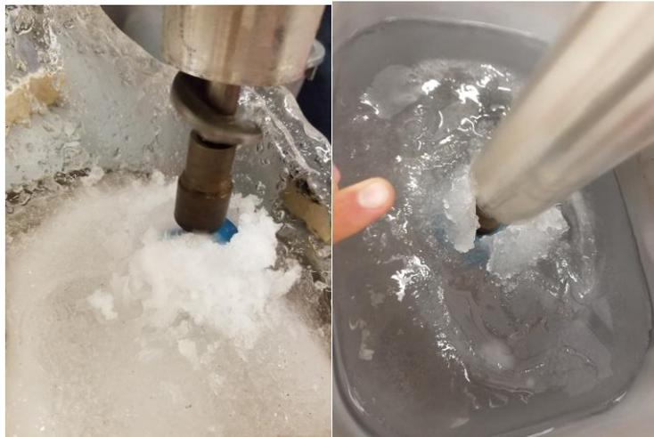
*Figure 11: IS-ICE entering the ice, as well as the lost ice chips on the surface of the sample.*
