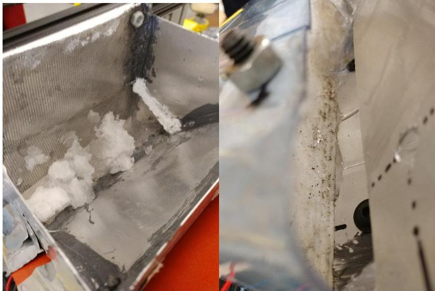
*Figure 4: IS-ICE Melt Chamber during systems integration test with ice only, and water filtering through 1-micron filter*
