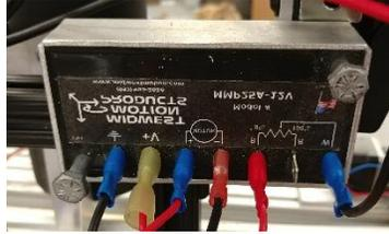
Figure 6: Drill speed motor controller
