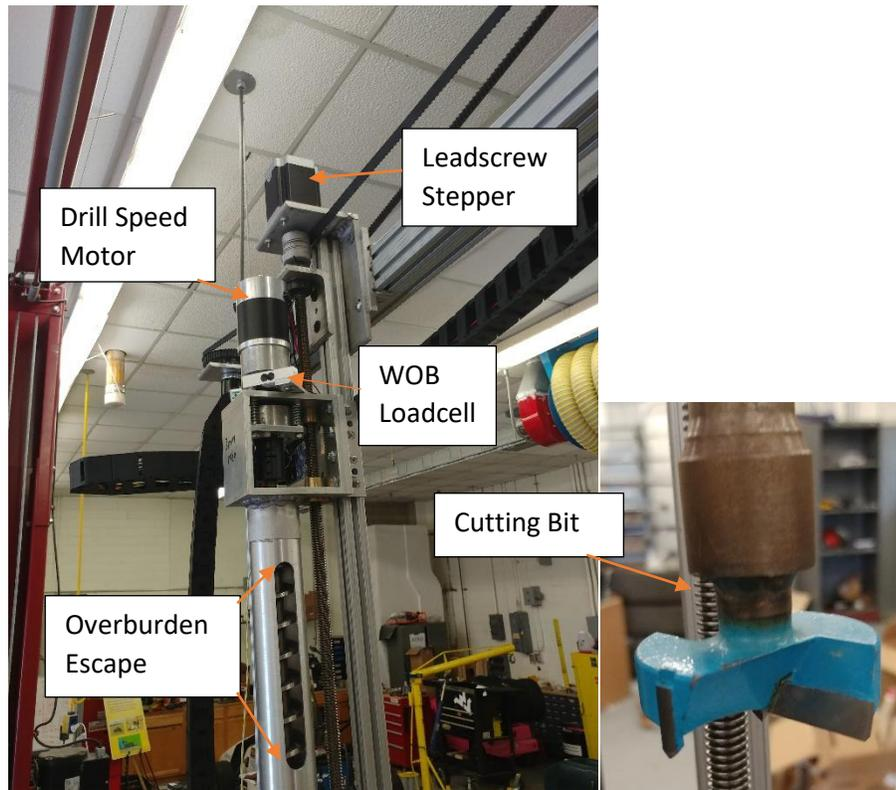
Figure 3: Drill motor mounting, load cells, overburden escape, cutting bit, and Y-axis motor
