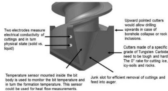
Figure 9: Example drill bit with conductivity sensors from Icebreaker drill.
