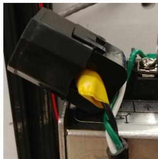
Figure 8: Over the wire current sensor
