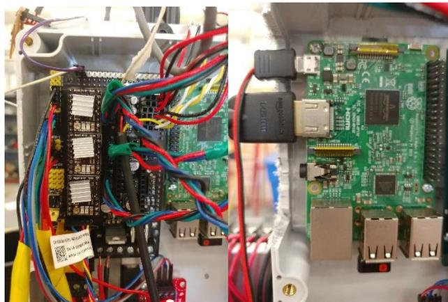
*Figure 5: Arduino with attached RAMPS 1.4 board and attached Pololu Stepper Drivers, and the Raspberry Pi 3*
