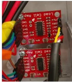
Figure 7: Load cell amplifiers
