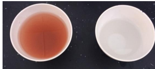
Figure 5: Clay Filled Water (left) and Filtered Water Using the Sawyer Filter (right)
