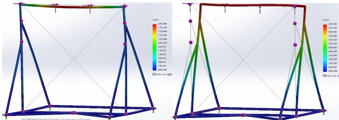
Figure 9: Stress Analysis on the Original Gantry Design
